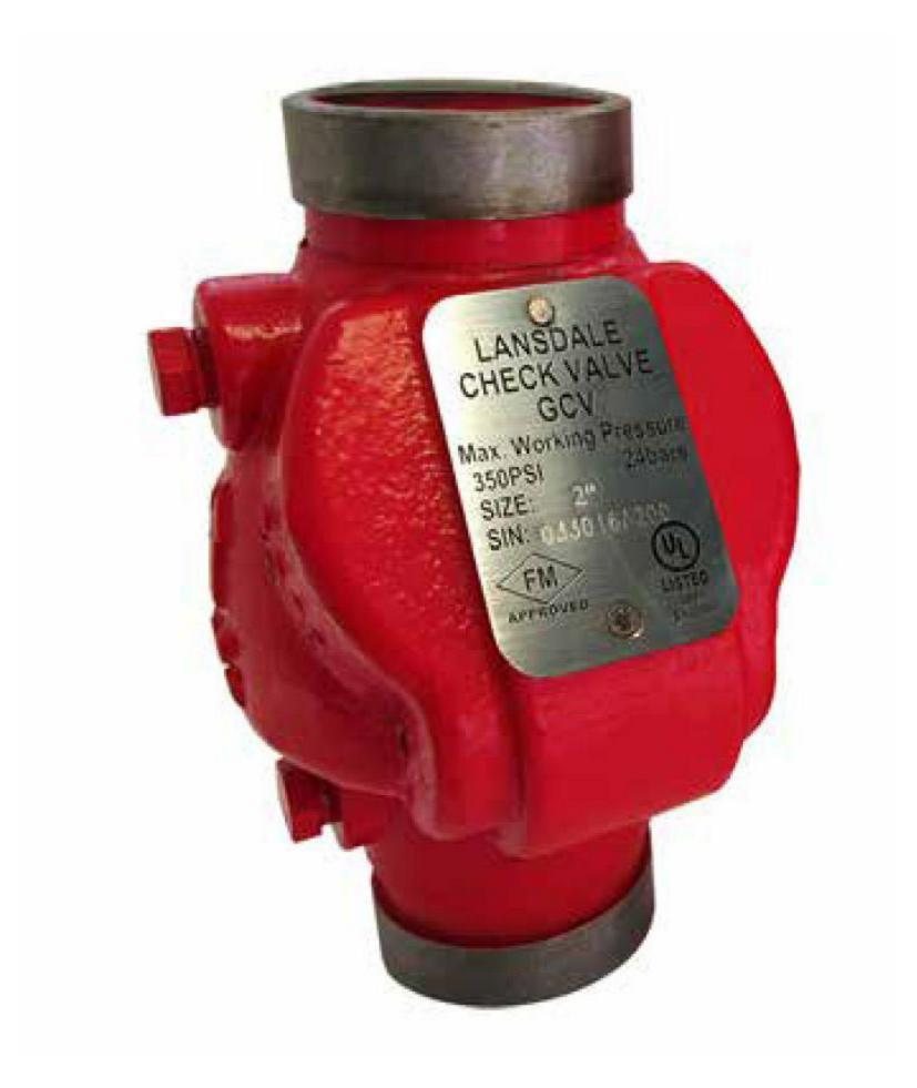
**Note:** Lansdale Check Valves may be damaged by excessively turbulent water flow. They should be installed a reasonable distance from pipe transitions, such as pumps, elbows, expanders, reducers, or similar devices. Typical piping practices suggest a minimum distance of five times the pipe diameter for general use.
